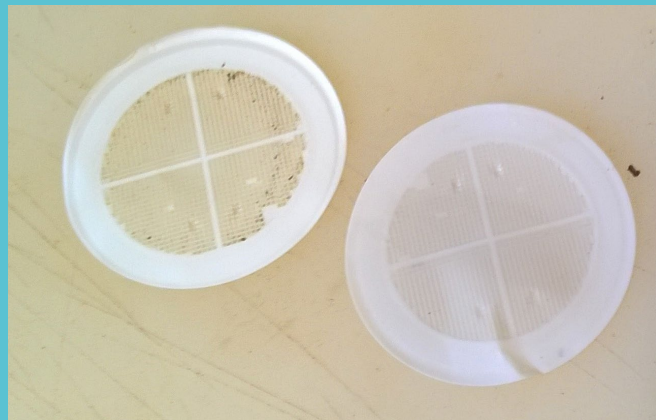
Well SDI pad on the left; taken at five (5) minutes into the flush.
