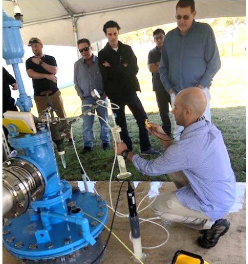
Field testing: Well performance data collection testing
